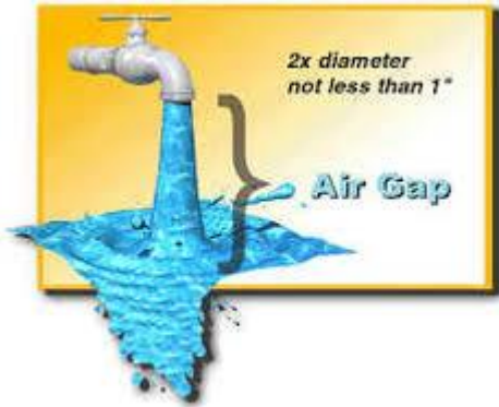
Air Gap Backflow Prevention
